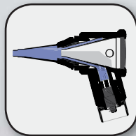
Fiber optics with 2.5V/3.5V XL xenon or 3.5V LED illumination ensure an unhindered, glare-free view.
