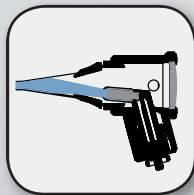
Reflection-reduced, cost-effective direct illumination with 2.5V or 3.5V XL xenon lamps.
